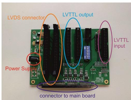
The breakout board provides the connectors for the various Bus systems. The LVTTTL inouts and outputs are connected to the digital input and output cards, which provide a galvanic isolation. The LVDS bus is connected to the DDS devices that provide an analog RF output.
